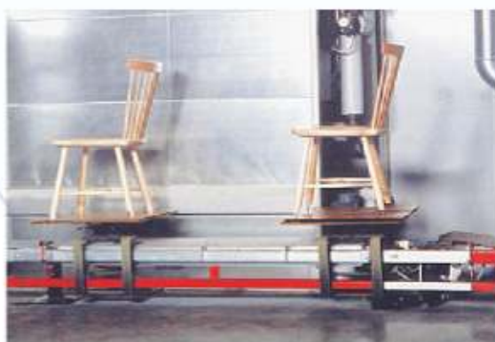
Floor conveyor (automatic varnishing line)
