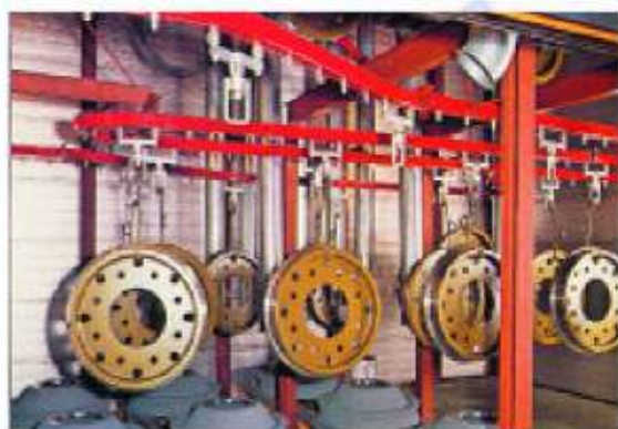
Overhead monorail chain conveyor (Foundry)
