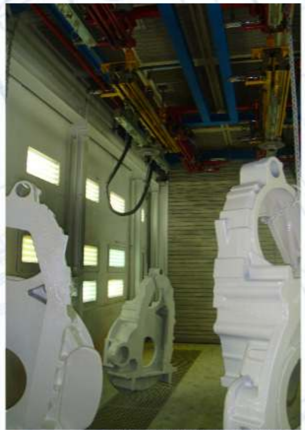
Elevator integrated in paint booth
